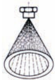
Hollow cone spray pattern
