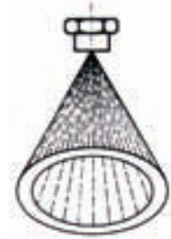
Hollow cone spray pattern
