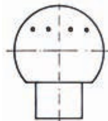
Type BD Ball with multiple jet, varies with request
